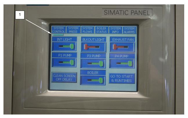
Figure 2. Selecting the System Control Display.
