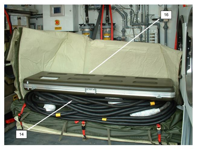
Figure 13. TEMPER light case on top of power cables.
