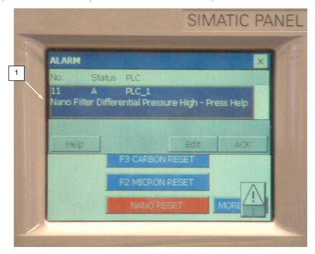
Figure 20. Nano Filter Differential Pressure High Alarm on PLC Display.
