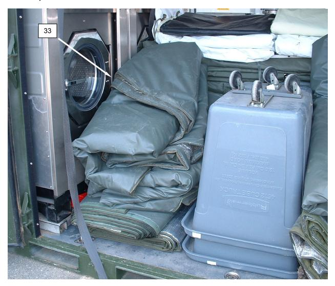
Figure 30. Place Second Set of Water Tank Insulation.
