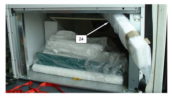
Figure 19. Placing the Water Tank Floats for Full Packout.
