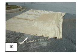
Figure 7. Prepare the 3000 Supply Water Tank for Movement.
