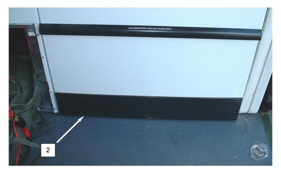
Figure 21. Installing Lint Compartment Door for Full Packout.
