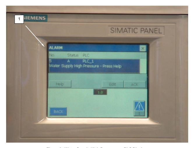
Figure 2. Water Supply High Pressure on PLC Display.
