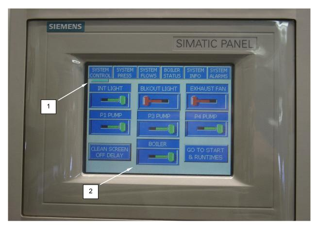
Figure 7. Operate the Boiler.
