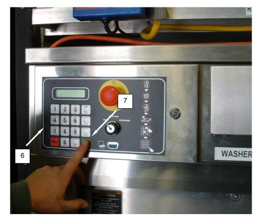
Figure 9. Nanofilter Cleaning Procedure - Start Cycle 59 on Washers.
