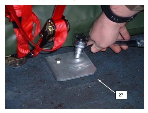
Figure 23. Install Retaining Brackets.
