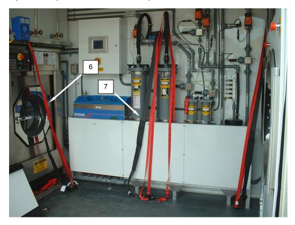
Figure 6. Attach Straps to D-rings.
