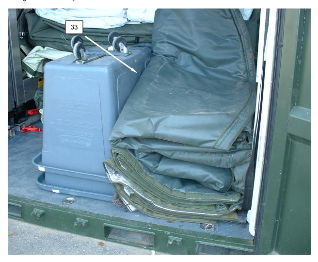
Figure 29. Place One Set of Water Tank Insulation.
