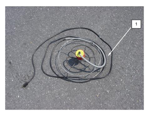
Figure 1. Tank Heater for 3000-Gallon Water Bag.
