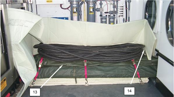
Figure 12. Placing the Cables for Full Packout.
