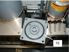
Figure 23. Replace the F-2 Filter Cartridge.
