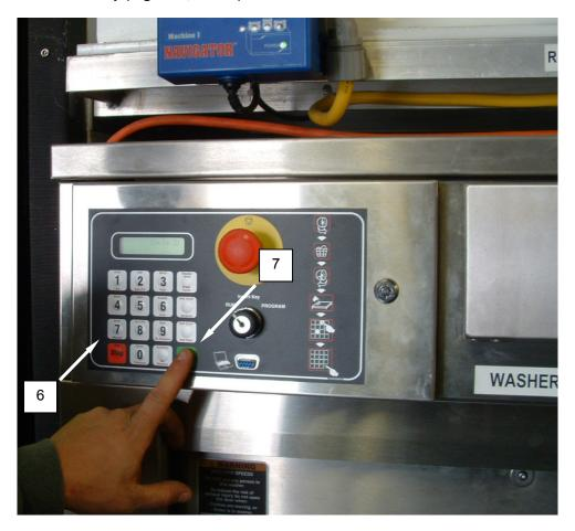
Figure 6. Nanofilter Cleaning Procedure – Start Cycle 70 on Washers.
