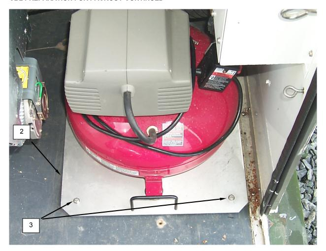
Figure 11. Pack the Air Compressor.
