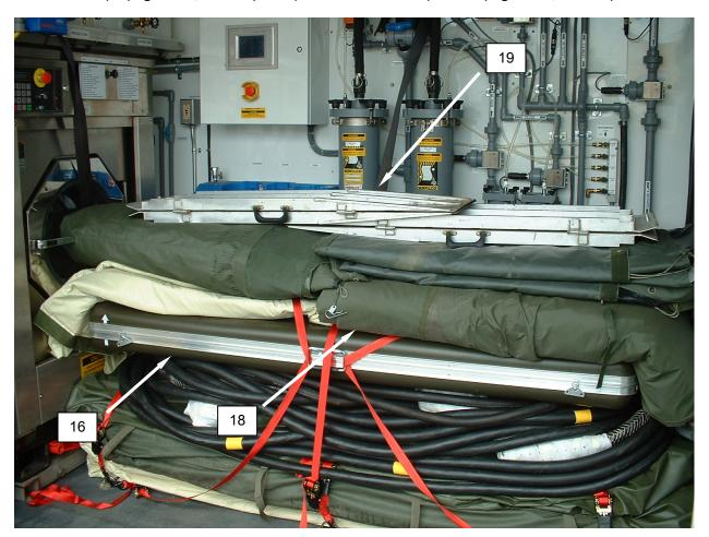
Figure 15. Placing the Ramps for Minimum Packout.
