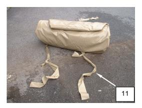
Figure 10. Prepare the 3000 Supply Water Tank for Movement.
