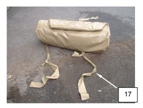
Figure 19. Prepare the 3000 Graywater Tank for Movement.
