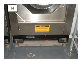
Figure 7. Open Soap Trays and Remove Kick Panels.
