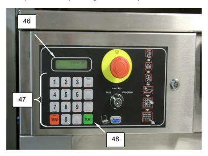
Figure 24. Washer Control Panel.
