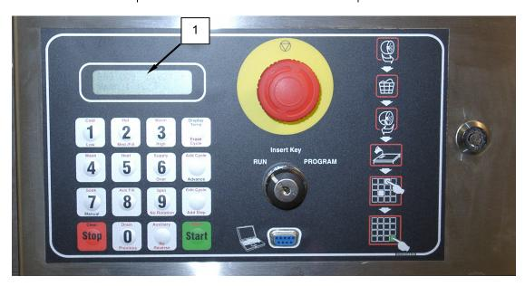
Figure 3. Didn't Drain Within Time Error on Washer Display.
