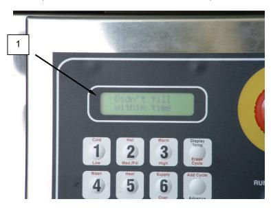
Figure 1. Didn't fill within time Error on Washer Display.
