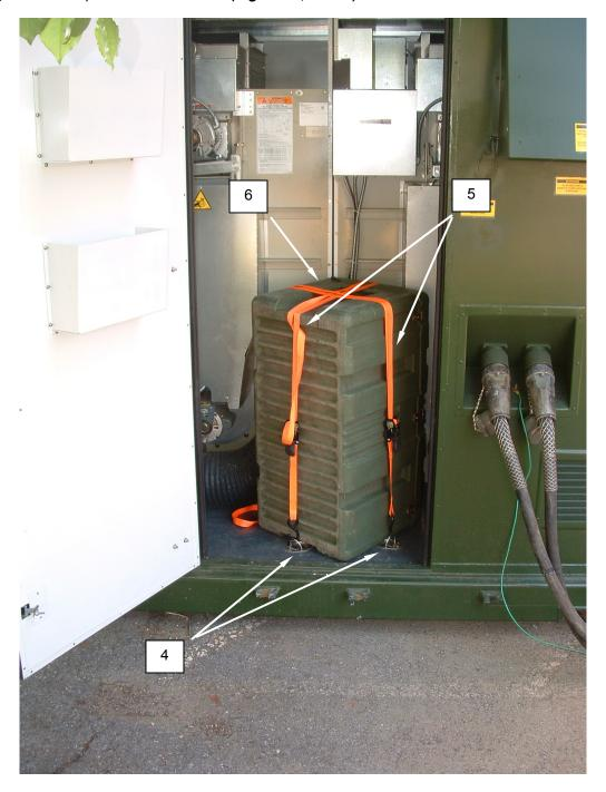
Figure 15. Pack the Footlocker in the CBL.
