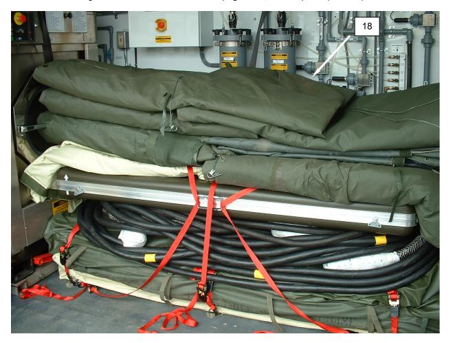
Figure 16. Outer TEMPER Fabric Sections on Top of Ramps.
