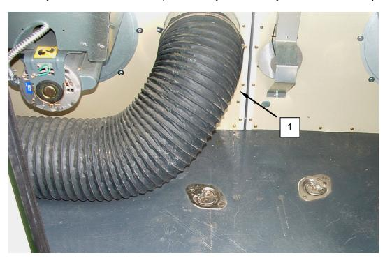
Figure 2. Clean the Dryer Exhaust Ducts.
