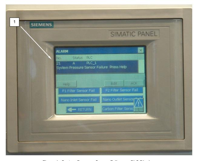
Figure 1. System Pressure Sensor Failure on PLC Display.
