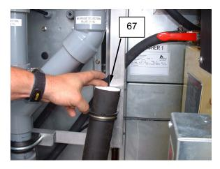
Figure 34. Add Antifreeze - Waste Water Tank.
