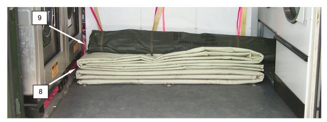
Figure 9. Packing Frame Section Bags.
