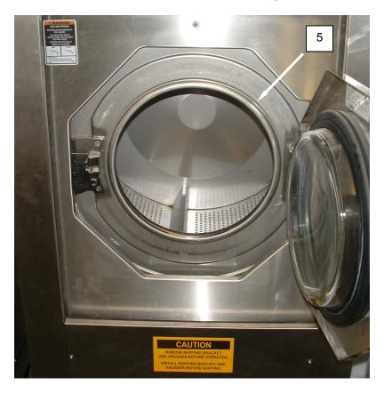
Figure 5. Nanofilter Cleaning Procedure – Add Chemical to Washer Drum.
