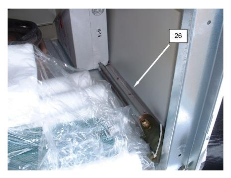
Figure 21. Fuel Can Adapter between Filters and the Dryer Cabinet.
