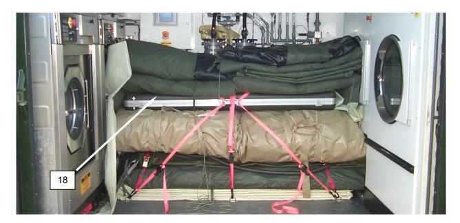
Figure 16. Placing the Fabric Sections.
