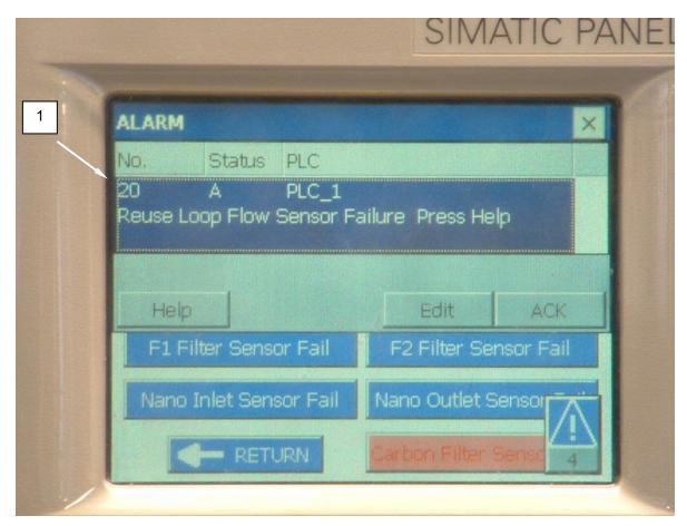
Figure 13. Reuse Loop Flow Sensor Failure Alarm on PLC Display.
