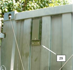
Figure 30. Close Container Vents during NBC Imminent or Actual Attack.
