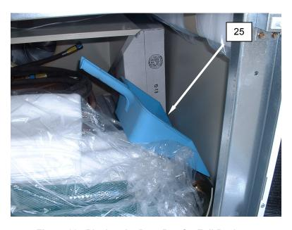
Figure 20. Placing the Dust Pan for Full Packout.
